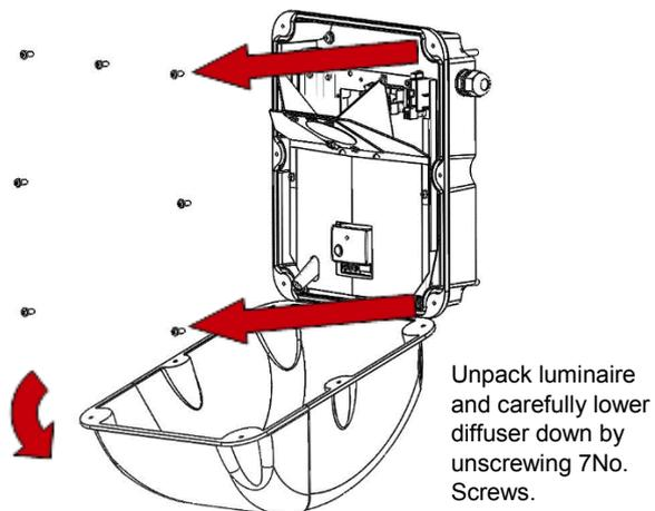
Unpack luminaire and carefully lower diffuser down by unscrewing 7No. Screws.
