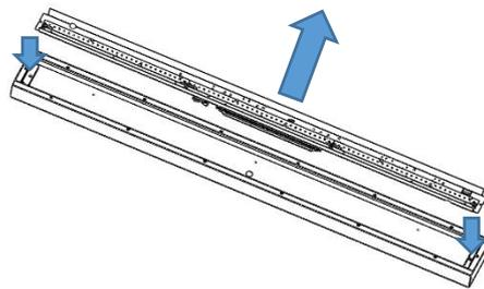
Unscrew the gear tray fixings at each end then remove the tray from the housing.
