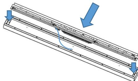
Wire the power cable into the chock block on the back of the gear tray. Then secure the gear tray back into the housing using the fixings at each end.
