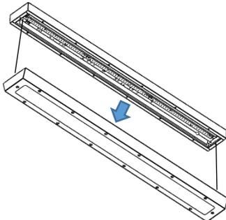
Remove the front frame and diffusers from the main body of the fitting. Allow the frame to hang from tether wires.
