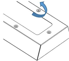
Undo the security fastener screws to release the front frame.
