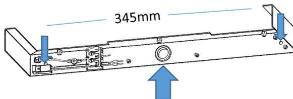
Then feed cable through the central hole and make the electrical connection to the terminal block.
