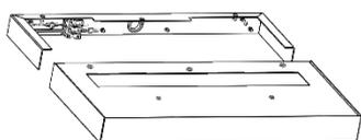
Connect the wall mount bracket to the fitting with the 2 pin plug and the earth cable to the brass tag.
