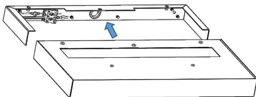
**4.** Screw the wall mount bracket to the wall using the two fixing points.
