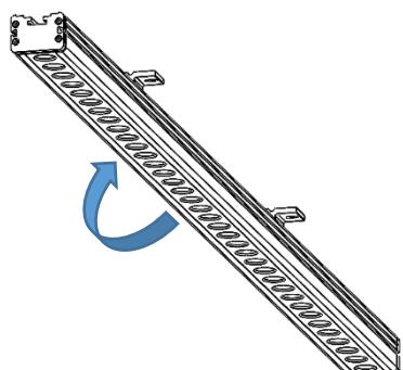
Position the fitting in the desired location and tilt to one side.
