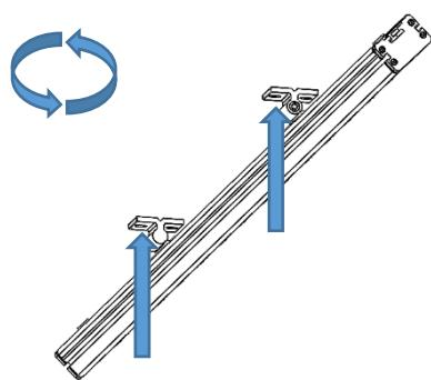
Rotate the fitting and fix the brackets on the opposite side.
