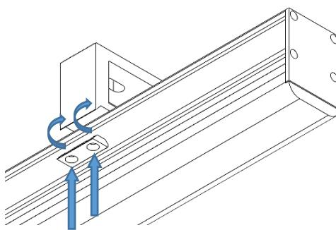
Reinsert the plate that was removed and secure in place using the screws provided.
