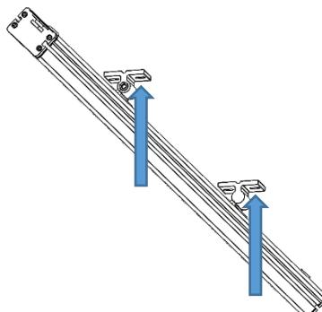
Fix one side of the brackets to the mounting surface.
