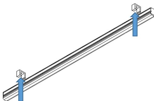
Offer the fitting up to the fixed brackets, and hold in place.
