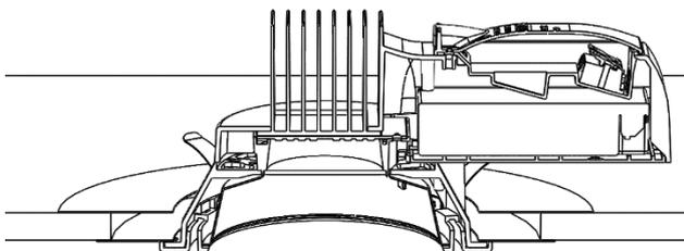
The downlight will need to be centralised in the ceiling aperture to ensure no gaps are visible.
