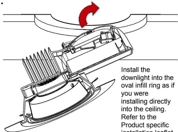
Install the downlight into the oval infill ring as if you were installing directly into the ceiling. Refer to the Product specific installation leaflet.
