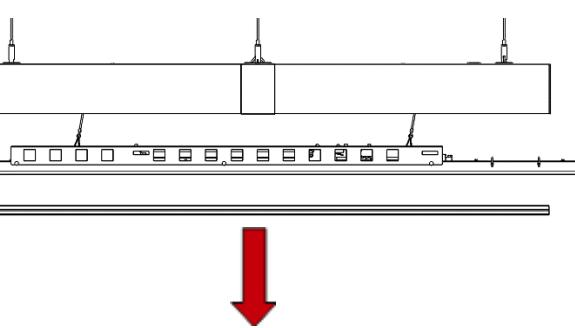
Remove the long 1200mm section of diffuser and drop the gear tray onto its tethers to access the starter bracket in the trunking.
