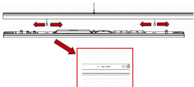
Slide tethers within trunking so they align with features on the fitting.
