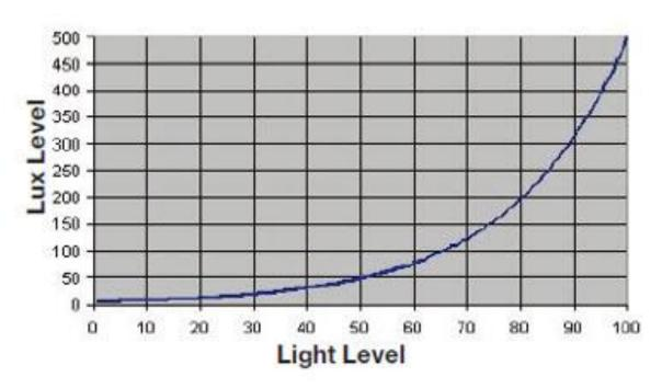
Lux calibration method (R24, R18, R44): This method provides accurate daylight regulation and also enables calibration of sensors during daylight hours where lux levels may exceed the required level.
