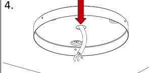
Feed the mains cable in through the drilled hole in the ceiling and through the base. Wire into the relevant terminals in the main housing and ensure the cable clamp is secured.
