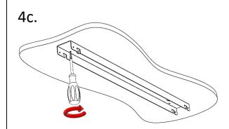
Surface mounted via 4x appropriate screw fixings into solid ceiling.
