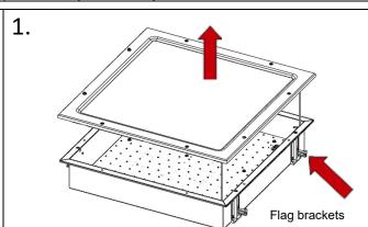
Remove diffuser by loosening each of the 8 retaining screws.
