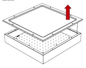
Remove and retain the 2 screws from the obround holes in the gear tray.
