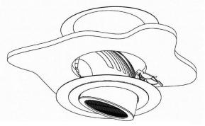
For installation into existing aperture greater than 174 (up to 220mm), use adapter ring kit.
