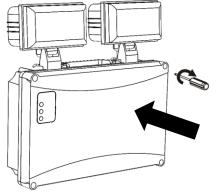
Refit the cover to the body, and secure in place using the four screws.
