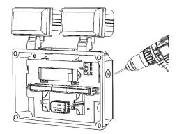
Drill the cable entry point on the side wall. Ensure the provided cable gland is fitted, to maintain the IP65 rating.
