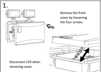
If required to remove gear tray, make sure to disconnect lamp head using plug and socket.
