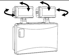
Rotate the heads to the desired position by loosening the screws accordingly. Be sure to tighten the screws once positioned, to hold them in place.
