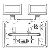
Pass the cable through the cable gland, and wire directly into the terminal block. Secure the mains cable using the internal cable clamp.
