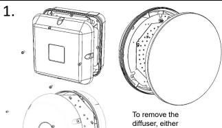
directly pull off (for snap-on diffuser) or remove screws to release the diffuser. 2.
