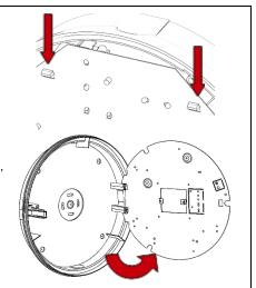
3. Drill a suitably sized hole in one of the designated places on the housing. The central Besa can be used as a cable entry if required.
