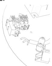
Wire the mains cable to the respective terminals on terminal block. Test the luminaire before reattaching the diffuser.
