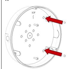
Attach the housing to the designated wall or ceiling with appropriate screws. Use the holes marked in housing.
