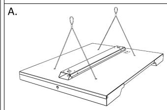
Suspend via 2x Y-fit wires (ordered separately). Do not suspend from single point!!
