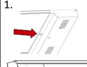
Remove 2x screw cover caps, then unscrew to release gear covers.
