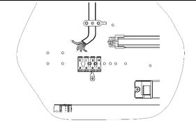
Connect incoming power cable as per diagram on leaflet. Use cable clamp kit provided.
