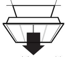
Isolate power supply then remove existing luminaire or ceiling tile.
