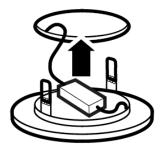
Place driver on panel, fold up spring clips and insert panel into ceiling
