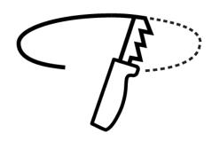
If no hole exists, cut 155mm (for 12W) / 209mm (for 20W) diameter hole in ceiling.
