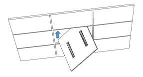
Lift and tilt the light fitting up into the ceiling void.
