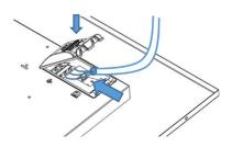
Wire the power supply into the terminal block. Then secure the back flap cover down to clamp the wire.
