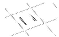
Drop the fitting down so that the front frame sits on to the ceiling grid. Installation is now complete.
