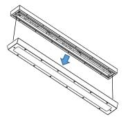
Remove the front frame and diffusers from the main body of the fitting. Allow the frame to hang from tether wires. 4.
