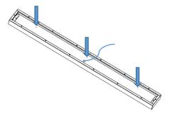
Feed the power cable through the central grommet hole. Then screw the housing to the wall using the 6 fixing points on the base of the housing.
