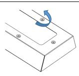
Undo the security fastener screws to release the front frame.
