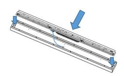
Wire the power cable into the chock block on the back of the gear tray. Then secure the gear tray back in to the housing using the fixings at each end.
