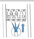
Make the electrical connection to the terminal block.
