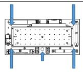
**Rectangular** – If mounting the fitting horizontally, cable entry hole to be in the 6 o'clock position. This will ensure that the emergency indicator is visible.
