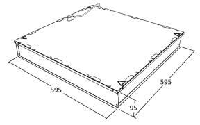
A minimum void of 300mm above suspended ceiling is required to install this luminaire.
