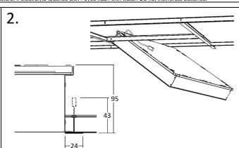
Remove ceiling tile(s), lift and rest fitting on T grid
