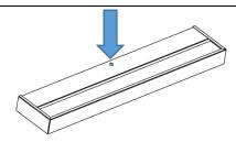
Fitting will be supplied complete. You will need to remove the wall mount bracket from the back of fitting in order to mount it to the wall. Remove the screw on the back edge of the fitting. This will release the wall mount bracket.
