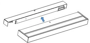
Slide the wall mount bracket out from the back of the fitting.
