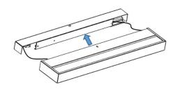
6. Sensor Version (Planum 500) – ensure sensor plug and socket cable is positioned in the channel between the driver and back of the bracket before sliding fully onto bracket.
