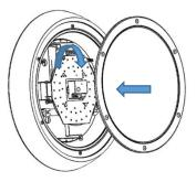
Flip the LED board back and secure in place using the fixing screw. Offer the diffuser and retaining ring up to the housing.
