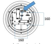
Bring power supply through central grommet and connect it to the terminal block. Then secure the housing to the wall using the 4 fixing points on the back side of the fitting.
