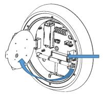
Undo the fixing screw in order to flip the LED board out of the way. This will allow access to the terminal block and fixing holes.
