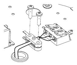
Use cable clamp and screws provided with fitting.
