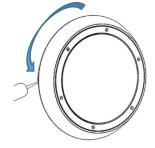
Run Anti-Pick Mastic around the profile of luminaire to ensure the fitting is secure. Must be installed with **anti-pick mastic** to meet ligature resistant requirements.
