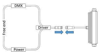
Connect the fitting to the driver. Then establish a connection with the free end of the cable.
