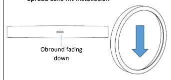
Ensure obround on spread lens kit is facing down to aid drainage.
