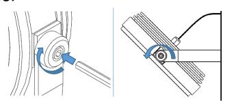
To adjust the angle of the bracket, use an Allen key to loosen the hex bolts on the sides. Retighten these bolts once at the desired angle.
