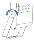
To adjust angle of the fitting, relax the 2 screws using an allen key.
