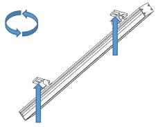
Rotate the fitting and fix the brackets on the opposite side.
