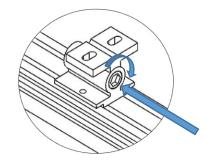
Once secure, position the fitting to the desired angle and then tighten the adjustable bracket on each end.
