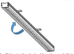
Position the fitting in the desired location and tilt to one side.
