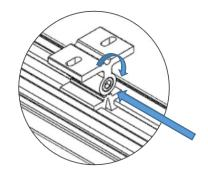
Once secure, position the fitting to the desired angle and then tighten the adjustable bracket on each end.
