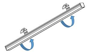
Packed with spring steel clips as standard. Secure these clips in the desired location.
