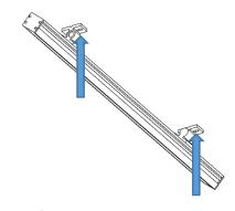
Fix one side of the brackets to the mounting surface.
