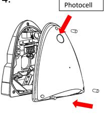
**Ensuring all** holes drill have been sealed to IP65, refit cover and fasten the screws. Fit cover caps in each hole in the orientation if the keys.
