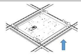
Regardless of ceiling type, the fixture should be offered up and into the aperture.
