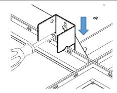
Each bracket should be adjusted, ensuring fixture is tight against grid/level with tiles where applicable - exposed T grid shown. Tighten screws on all brackets.
