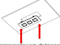
Once electrical connection is made, offer fixture in to aperture. Retract 2No adjacent springs - fit in ceiling retract remaining 2No springs to complete installation
