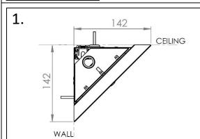
X-section through fitting – note that fitting should be mounted with dimpled fixings to ceiling!
