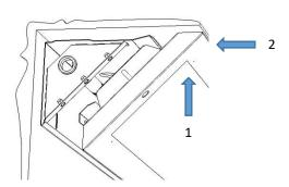
Cover should be pushed to ceiling first (1) and then forced on to the main housing (2) – this will grip the cover prior to securing with screws
