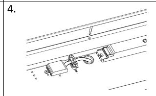
Electrical feed can come through central hole (shown) or through the end plate. Use cable clamp kit provided.
