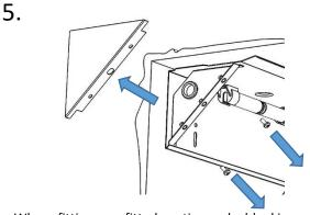
Where fittings are fitted continuously, blanking end covers must be removed (leave in place for start and end of runs)
