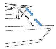
When offering up front LED cover, make sure cable is connected between the two sections! Ensure earth lead is also connected to frame!
