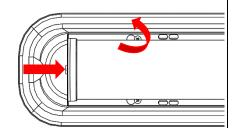
Loosen all 6 screws and slide the gear tray to release it from the body.
