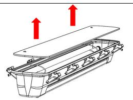
Remove front cover (cover is retained on 2No wire hangers)
