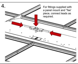
Once electrical connection is made, offer luminaire into ceiling aperture diagonally and rest on rear face of ceiling T grids – be sure to check it sits
