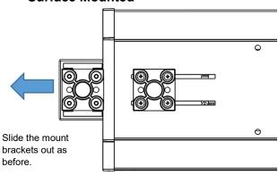
Using the two black plastic spacers provided, secure the fitting directly onto the surface using 4x suitable screws each end (not provided).
