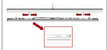
Slide tethers within trunking so they align with features on the fitting.
